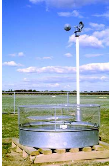
Figure 1 Class A Evaporation Pan
